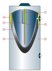
cold water in the tank is passed through solar collectors, where it is heated before returning to the top of the storage tank. Electrically-boosted solar systems include an integrated heating element.
